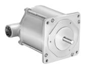
The explosion-proof MX Series provides hazardous-duty stepper motors suitable for use in Class 1, Division 1, Group D locations. They are available in NEMA 34 and 42 frame sizes (90 and 110 mm), and provide minimum holding torques from 1.27 to 9.82 N-m (180 to 1390 oz-in).
