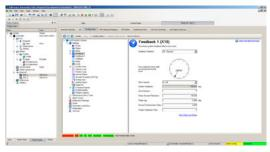
Complete motion system configuration from one location with embedded AKD Workbench allows configuration of all servo drives over EtherCat®.
