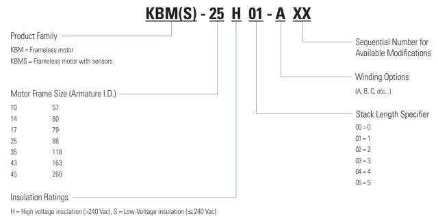
Note: H insulation is standard option for frame sizes 10, 14, 17, 25, 35 and 45.
