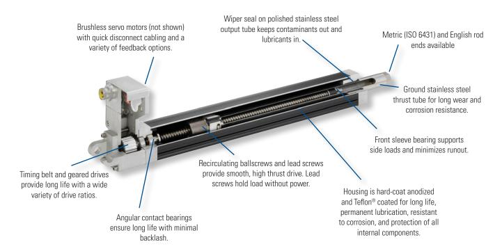
**Kollmorgen offers electric cylinder drive mechanisms designed around either lead screws or ballscrews.** Ballscrews, being the more efficient of the two, utilize ballnuts riding on recirculating ball bearings resulting in higher speeds, loads and cycle rates. However, the more efficient design of ballscrew technology lends it to being backdriven when power is removed if precautions are not taken (e.g., electric brakes or counter loading).
