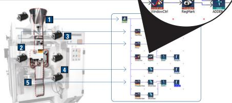
Pipe Network provides a one-to-one translation of a mechanical system into a logical world as shown in the Vertical Form Fill and Seal machine above. Click and build your motion program in minutes, or contact Kollmorgen for examples of common machine architectures to further accelerate your development.
