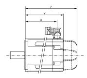
Measure Y: Without holding brake Measure Z: With holding brake
