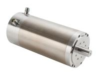
These brushless servo motors incorporate pressure compensation technology to allow underwater operation up to 20,000 ft while withstanding extreme environments. They feature stainless steel and aluminum nickel bronze housings or an anodized aluminum housing for lighter overall weight. All shafts are stainless steel and sealed with an externally serviceable 0-ring seal. The S Series is fully tooled for cost-effective volume production.
