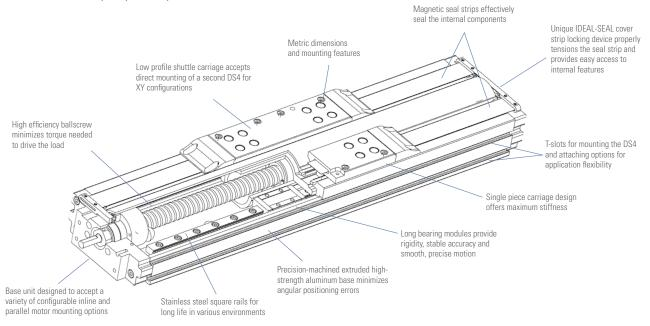
DS Series precision tables can be ordered in a variety of multi-axis configurations including XY, XZ, and XYZ or cartesian arrangements. Consult Kollmorgen applications engineering for standard and custom configurations.
