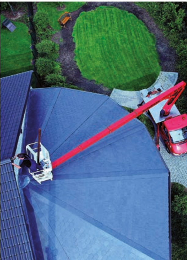
When positioning a sky lift basket, using smart actuators makes it possible to limit movements and avoid potential dangers.
