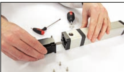
Insert motor shaft into coupling
