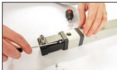
Tighten motor mounting screws
