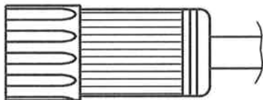
Shield connected to metallic cover
