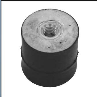
Vibration damper Internal M8 both sides SH 65 A Ø 30 x 30 mm
