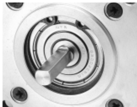
Two flats on drive shaft permit use of dual setscrews for increased locking force.
