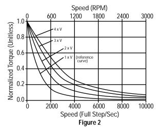
**Figure 2** shows the performance of the same motor driven by a bipolar chopper driver with different supply voltages. All drivers have the same current setting. Note that low speed running torque is not appreciably affected by supply voltage differences. High speed performance, however, varies considerably with changes in supply voltage. Caution must be exercised when increasing supply voltage as higher voltages will result in increased motor heating.
