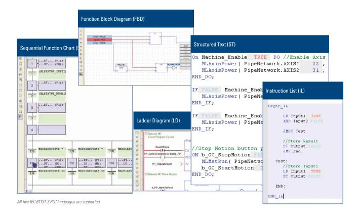
• Kollmorgen Automation Suite's integrated development environment (IDE) allows the developer to create solutions without having to connect a single device by using the offline simulator. Start creating systems before the first hardware component is delivered. Simply configure your system network in "offline development" mode and change the status of the devices one-by-one when you actually connect them.
