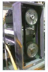
Press feed machine built with a conventional servo motor, gearbox, belt and pulleys.
