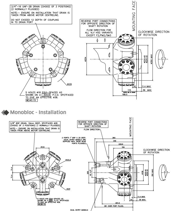
DUAL ENTRY MODELS: 2 SIDE PORTS 1" BSP x 25 DEEP. SPOTFACED TO \$63.
