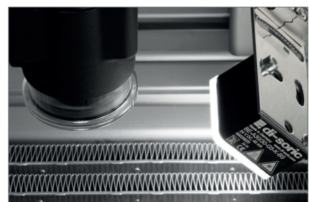
Produktkontrolle mittels Vision Sensor und Auffichtbeleuchtung (BE-A30/30-G5-K-BS) Product monitoring with a vision sensor and barlight (BE-A30/30-G5-K-BS)
