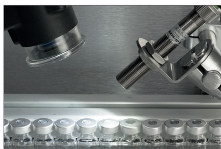
Verschlusskontrolle mittels Vision Sensor und Punktbeleuchtung (BEK-PM12-G5T-BS) Detection of missing caps with a vision sensor and spotlights (BEK-PM12-G5T-BS)
