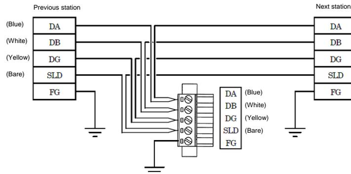
Fig. 2.5 Connection example of communication cable
