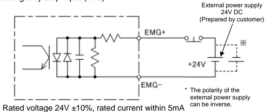
Fig. 2.6 Connection example of emergency stop input (TB3)
