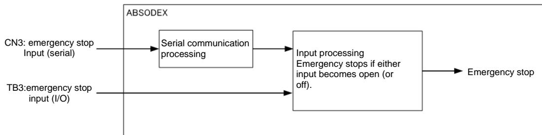
Fig. 2.7 Specification of emergency stop input
