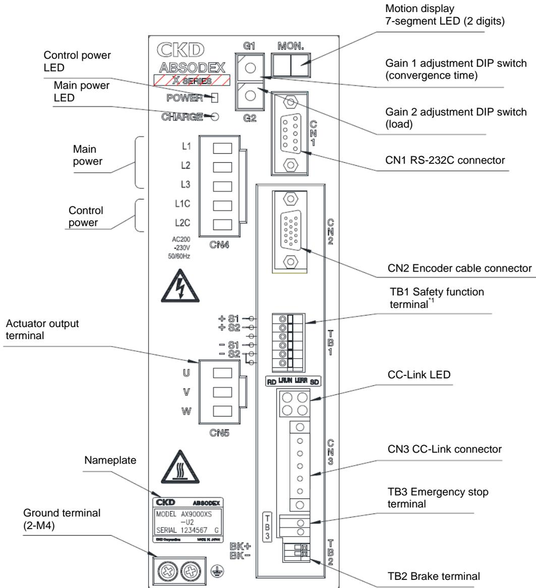
Fig. 2.1 XS type CC-link specification, Driver panel
