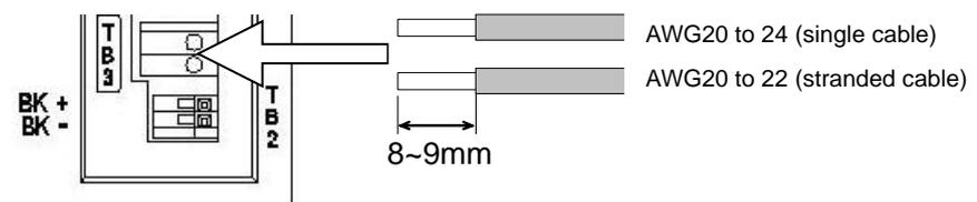
Fig. 2.8 Applicable cable to TB3 and peeling size
