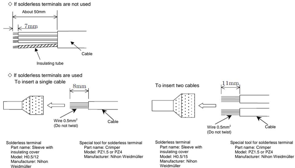
Fig. 2.4 Peeling size of communication cable
