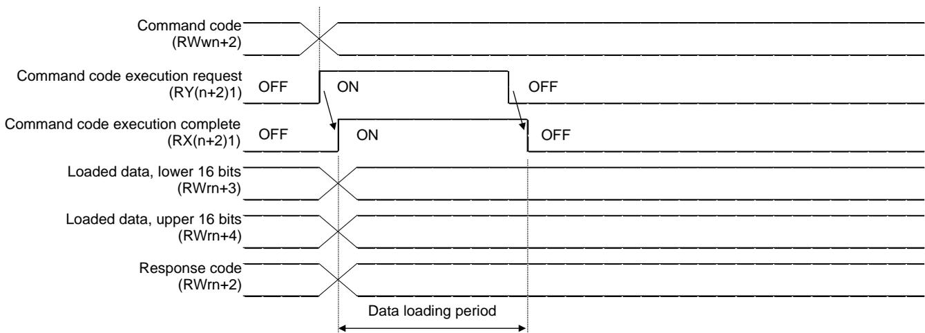
Fig. 3.2. Timing chart for load command code execution
