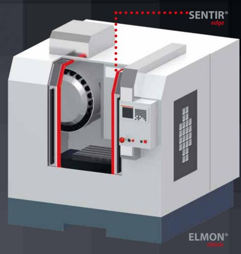
Safety contact edges are pressuresensitive sensors that are used as protection against entrapment, for example - on automated gates, AGV's, machines and handling devices or movable stage elements.
