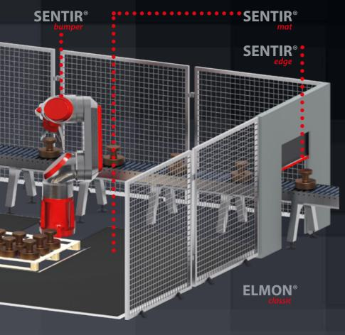
Safety relays are used for connecting **SENTIR** tactile safety sensors and the PLC. They ensure a continuous monitoring and evaluation of the safety sensor.
