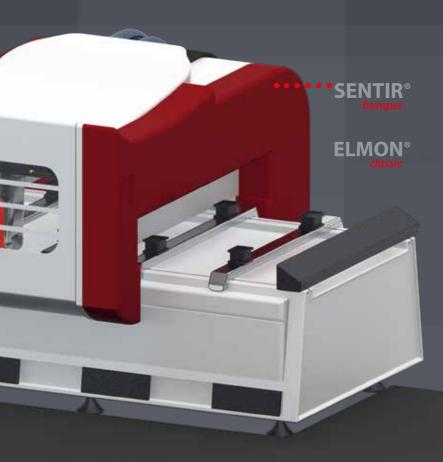
The **SENTIR** safety contact bumpers provide excellent cushioning and overtravel. They protect the operator and offer safe interaction between man and machine due to their limited space requirements.
