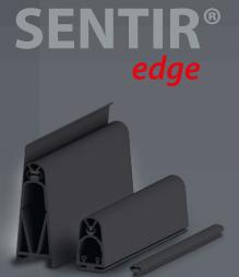
**SENTIR** *edge* safety contact edges are pressure-sensitive sensors for closing edge protection, with optimum overtravel distances and extremely fast switching behaviour. The Plug'n'Sense self-assembly system makes it possible to assemble a safety edge without tools or glue within a very short time and independent of ambient conditions, e.g. when servicing is required directly at the door. **Simple. Safe. Unique.**
