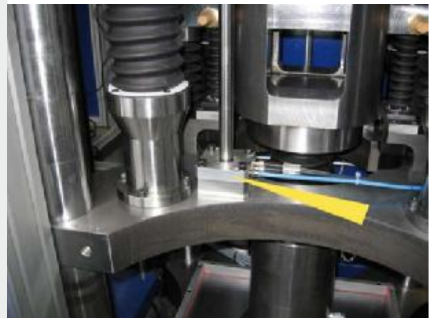
Pneumatic rod clamping allows hydraulic presses to be used for any application KOMAGE Gellner Maschinenfabrik KG, 54427 Kell am See, Germany
